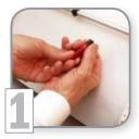
Adjust Blade. You can dial out the exact depth of knife blade to make the perfect cut.
